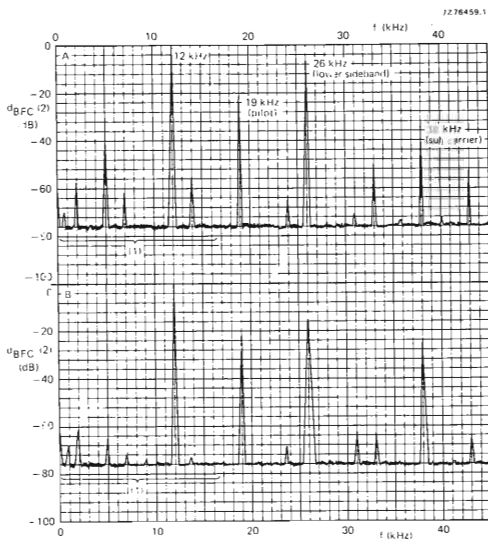
(1) Audible interferences (BFC distortion) and undesired 12 kHz signal.
