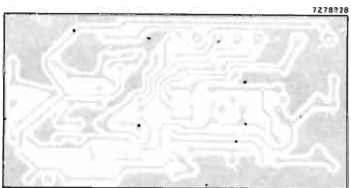
Fig. 12 Printed-circuit board showing track side.
